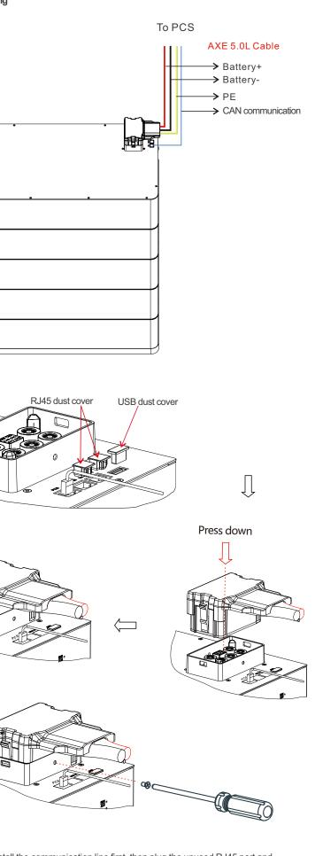
**Note:** 1) Please install the communication line first, then plug the unused RJ45 port and USB port with a dust cover, and finally install the power line. 2) No cable connection required between battery packs in a single battery cluster.
