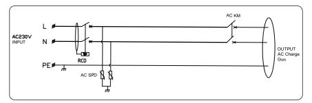
Fig11-1. Main circuit diagram
