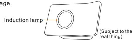
**Induction lamp status:** Flashing red: Network configuration status
