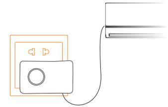
After the first power-on, the indicator will enter the red flash status. If not, press and hold the reset button.
